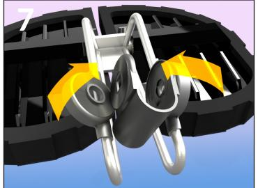
Squeeze the post clamp and the second inner clamp together until they snap into each other. Be careful not to pinch your fingers!
