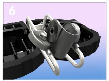
Put the groove on the inner clamp on the front edge of the triangle shaped bar.
