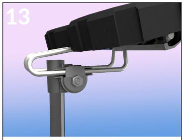
With mount nuts loosened slide the seat until the mount is near the midpoint of the triangle rails.
