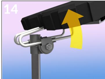
Tilt the rails so they are positioned at a slight downward angle and tighten the nuts on the mount to secure the seat's position. Test ride the bike.
