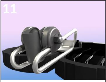
Place the second outer clamp onto the other end of the bolt and thread the second nut onto the bolt.
